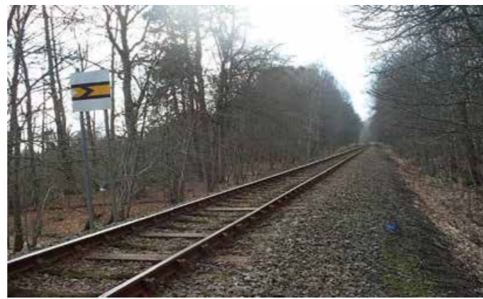
Figure 11 – Fixed distant Board
