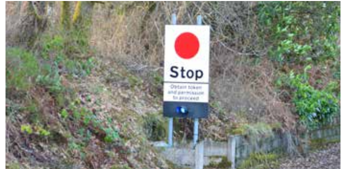
TRCU Lineside Status Indicator
